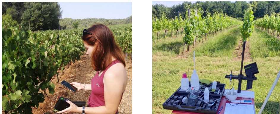
Figure 4 pictures showing measurements on wine leaf with NIR scanner (left) and electro-chemical test set (right)
