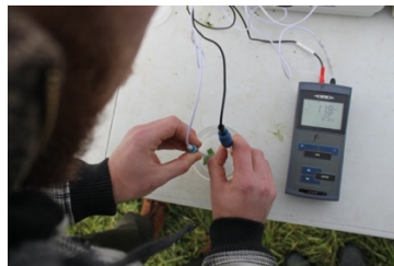
Figure 2: Measuring redox potential in the field with traditional electrochemical method
